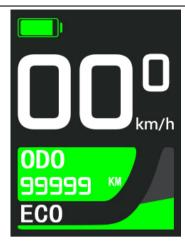
Real-time speed and Odometer display
